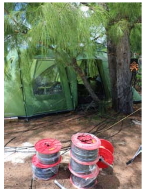
We used 1,500 meters of low-loss coaxial plus an additional 500 meters of 75 ohms coax for receiving antennas.
