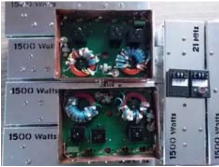
Perfo Box 1500 bandpass filters and four square relay switch units.
