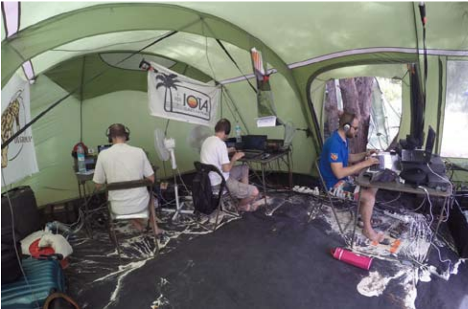
Inside one of the tents with the same setup — radio, laptop, amp and interface — for each operating position.
