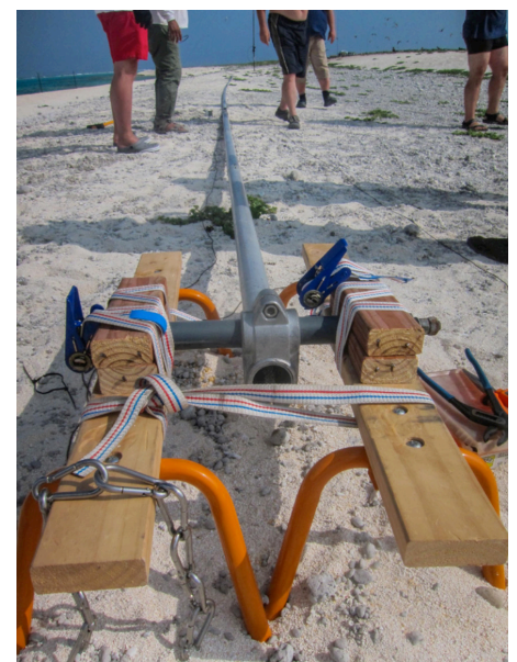
Titanex vertical with a homemade 160M base constructed from two sawhorses, straps and 2x4 boards.
