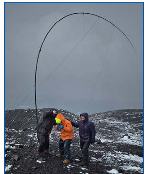
In heavy wind gusts, the guys could hardly stand upright and the 80M full-size vertical bent against the winds.
