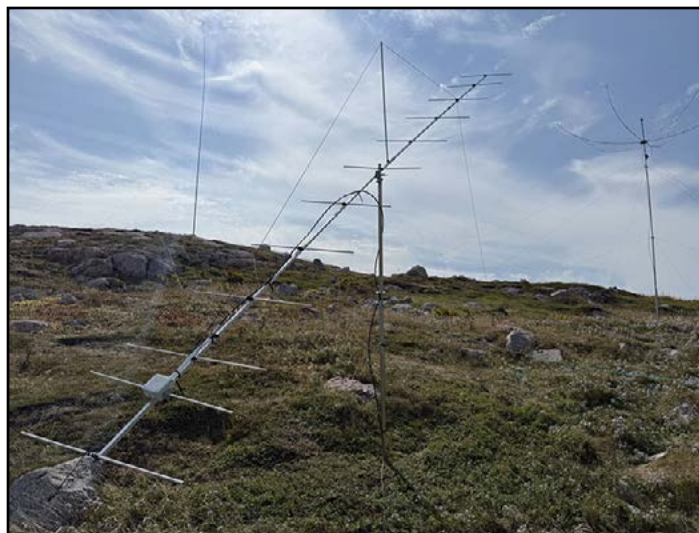
Left: 160M top loaded vertical antenna. Right: 12-element 144 MHz homemade Yagi for EME.
