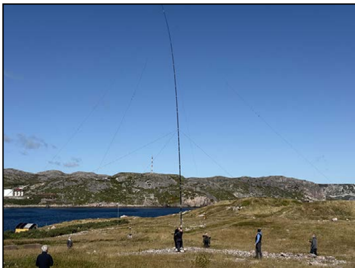
Left: 160M top loaded vertical antenna. Right: 12-element 144 MHz homemade Yagi for EME.
