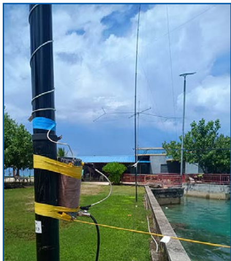
160M antenna with a loading coil.
